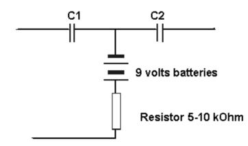
C1 and C2 will, if the battery voltage is chosen high enough, never reach zero voltage, where the memory effect comes forward. It is a cheap trick for you to try.
